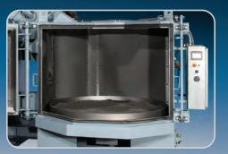
**Powered Turntable** rotates parts within the blast stream for even exposure.
